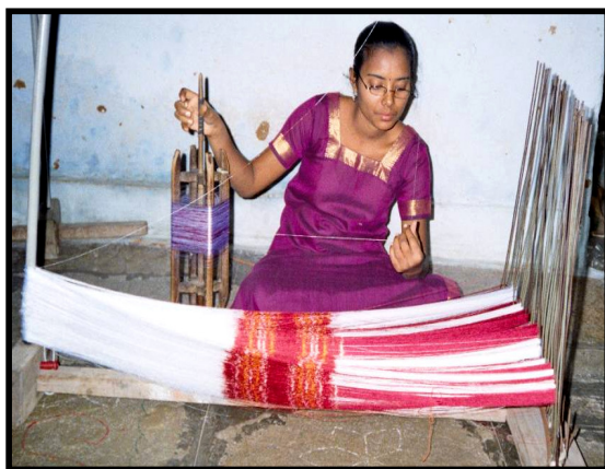
Reeding the warp yarns and weft yarns
