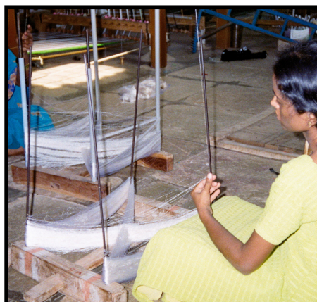
Reeding the warp yarns and weft yarns
